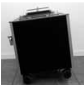
Side view of multifunctional boiler with tilting mechanism.
